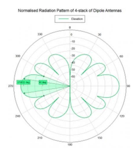
The second antenna would use half the number of antenna elements and will have a gain of nominally 3dB less than the first.
