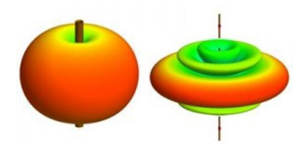
Looking at the above radiation patterns, it should be noted that a single dipole has a radiation pattern with a wide beam and gain of about 2.2dBi. The second figure shows an array of four dipoles identical to the first.
