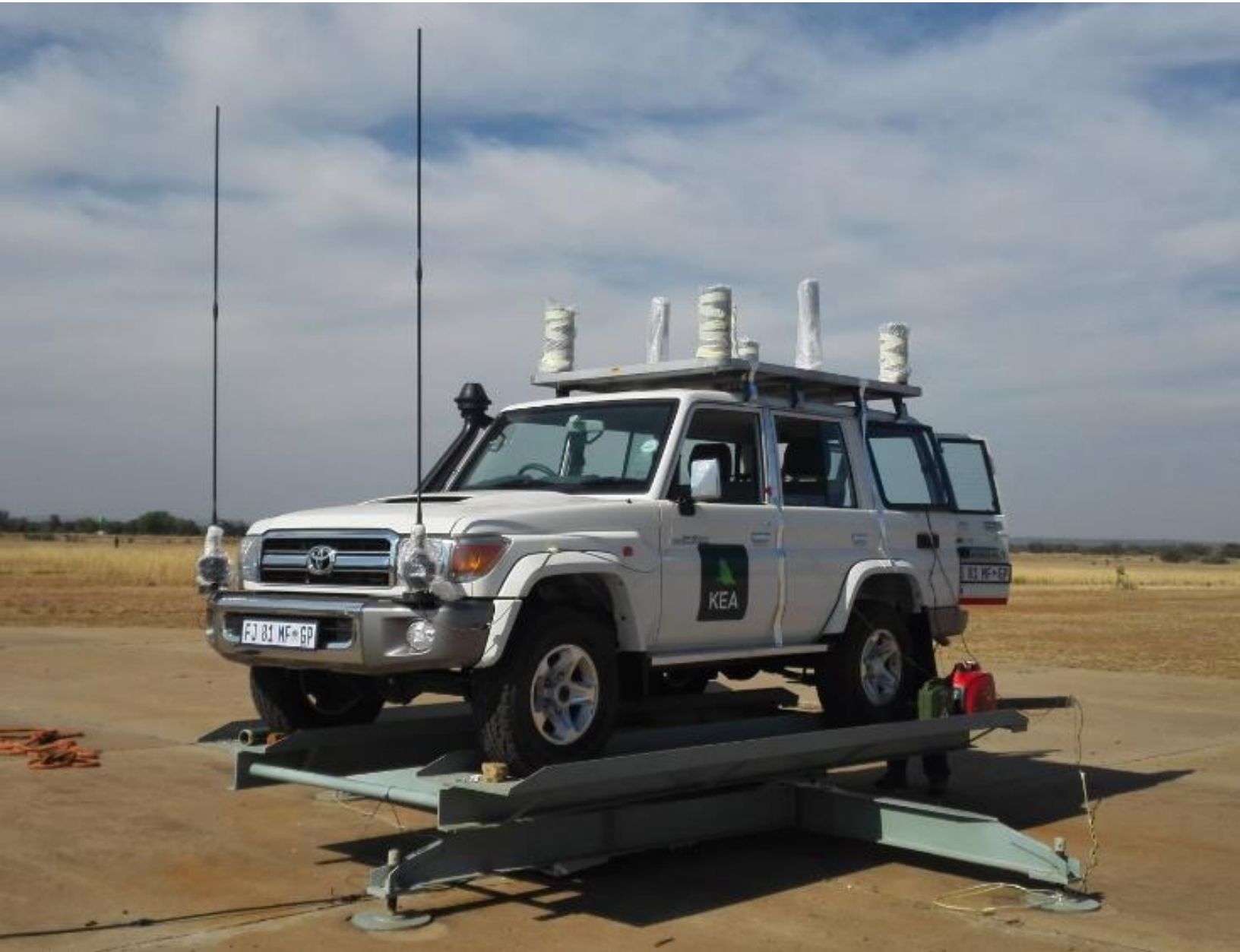
Figure 2. A vehicle with two whip antennas (MONO-A0062) on the front corners of a vehicle being measured. The other antennas on the roof (OMNI-A0281, OMNI-A0266) are all dipole-type antennas.
