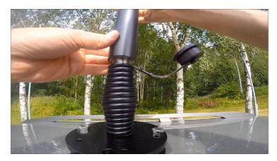
Figure 1 - Removable dipole radiator mounted onto a vehicle
