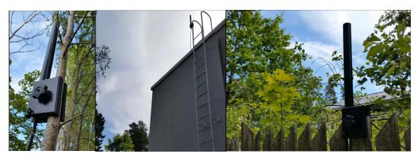
Figure 2 - Removable dipole radiator attached to a Mast
