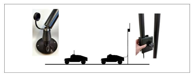
Figure 3 - Vehicle installation (Left) and Mast installation (Right)
