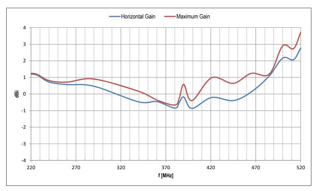
Figure 7 - Antenna gain (Mast installation)
