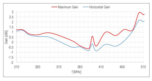
Figure 8 - Antenna gain (vehicle installation)
