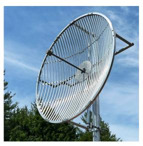
The mWAVE Mark Compak grid reflectors ship in 4 pieces for ease of handeling on site and shipping. The antennas have the same performance as their single piece counterparts.
