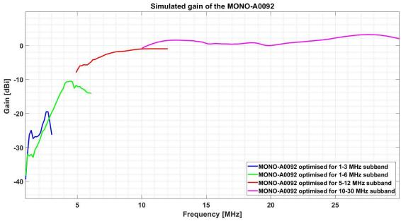
Figure 2: Antenna gain in untethered configuration
