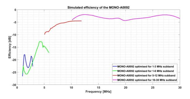
Figure 3: Antenna efficiency in untethered configuration
