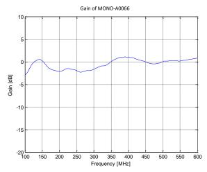
\*\*On horizon, on a typical vehicular groundplane
